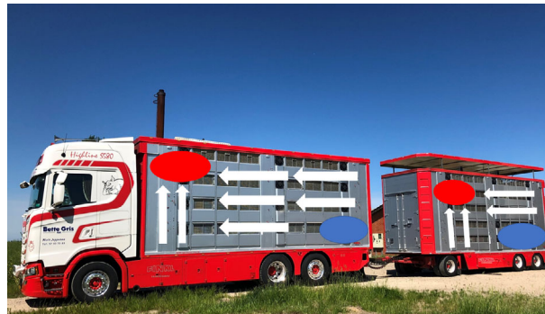
Figure 7: Predominant patterns of air flow (black arrows) in a moving passively ventilated vehicle. Red areas indicate where air heated by the animals accumulates and blue areas show colder spots. Photo: Marianne Kaiser, Aarhus University
